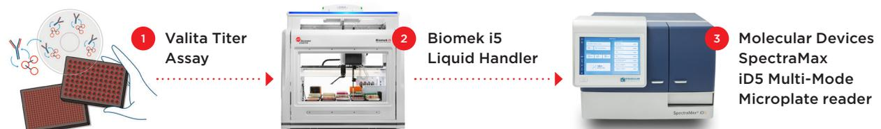
**Figure 1.** The technologies used in this work to acquire high-throughput IgG quantification. 1) The Valita Titer IgG quantification assay plate; 2) The Biomek i5 liquid handler, responsible for standard curve creation and plating of standards and samples; 3) Molecular Devices SpectraMax iD5 reader, which performed FP measurement on the Valita Titer assay plate.
