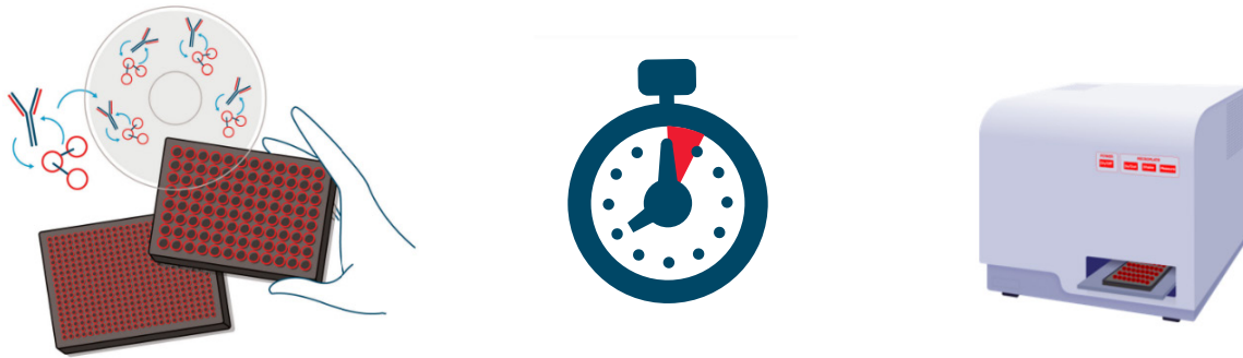
FIGURE 2. Workflow schematic of Valita Titer assay. 1. Add fresh media and IgG sample and mix. 2. Incubate for 5 minutes at room temperature. 3. Measure IgG using fluorescence polarization on a plate reader.
