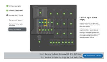
Figure 16. Teardown Procedure with Cold Storage 3 position highlighted on the Deck Diagram.
