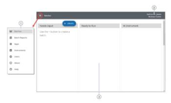
Figure 6. DBiomek NGeniuS Portal Software User Interface with the Main Menu (1), the Active User Information (2) and the Workspace (3) highlighted.
