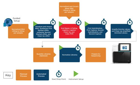
Figure 1. The Illumina TruSight® Oncology 500 DNA/RNA Automation App Template Workflow.
