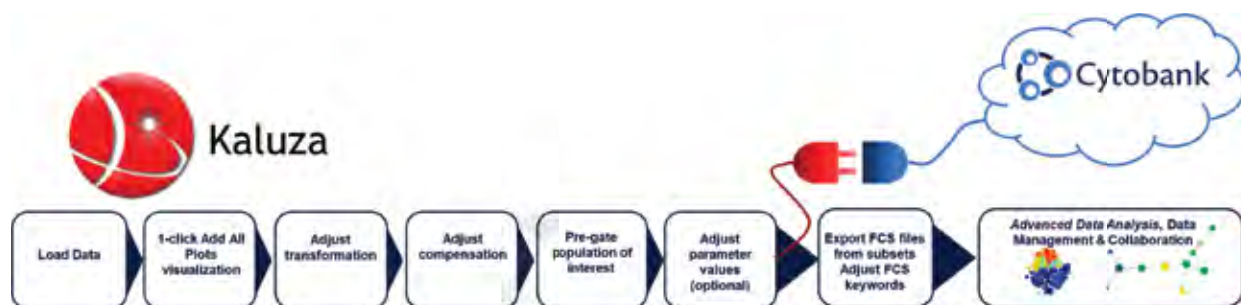
Figure 1: Steps in the flow cytometry analysis pipeline covered by Kaluza and the Cytobank platform. The Cytobank platform offers automatic compensation calculation but manual adjustment of the compensation matrix is more interactive in Kaluza. Gating steps on biaxial plots work well in both systems. For exploratory data analysis, clustering and data visualization Cytobank is the software of choice.
