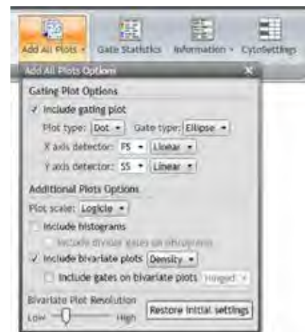
Figure 5: Add All Plots Options selections used for the example shown here. Include gating plot with plot type: Dot and Gate Type: Ellipse, chose FS Linear and SS Linear as X axis and Y axis detectors, respectively.
