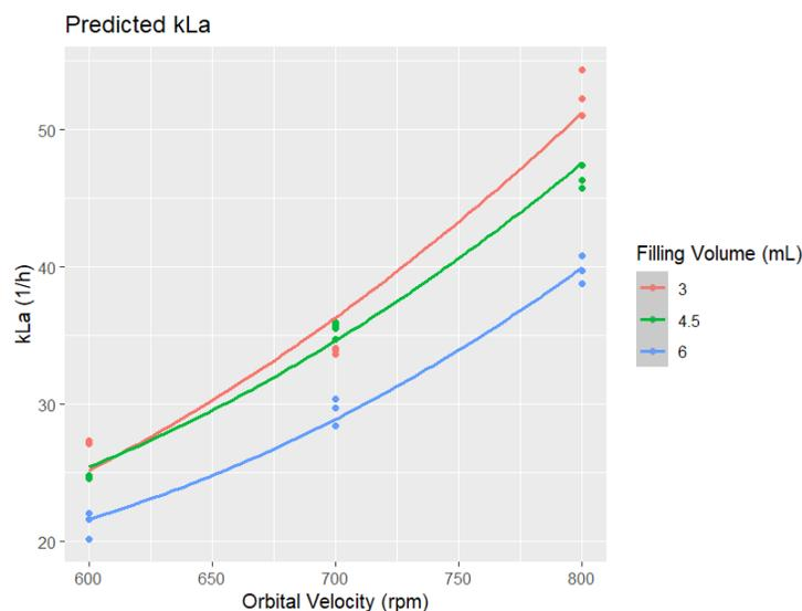
**Figure 3.** Prediction of  $k_{La}$  overlaid with experimental measurements.
