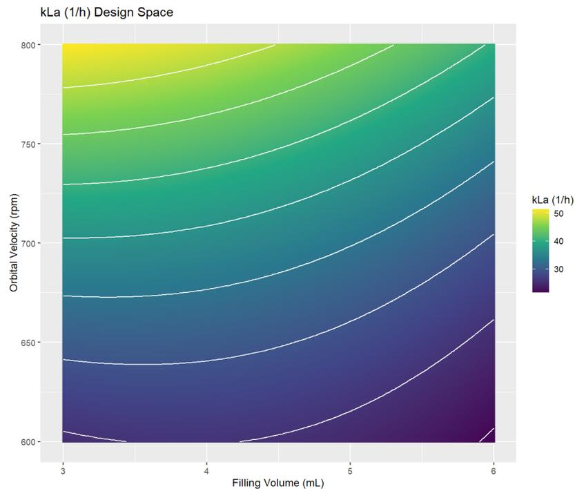
**Figure 2.** Dependency of  $k_La$  on shaking frequency and filling volume.
