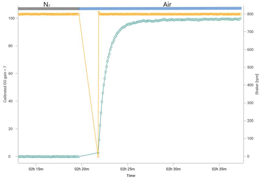
**Figure 1.** Dissolved oxygen saturation curve (green) during a  $k_La$  determination experiment. The shaker (yellow) was stopped briefly after air gassing was started to flush the headspace.
