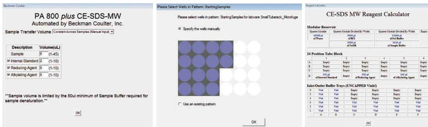
**Figure 3.** User Interface Screenshots. A) The user interface allows the selection of reagent and sample volumes and (B) sample locations using either a runtime pattern or a worklist file. C) The reagent calculator shows the location and total reagent volumes required, as well as the buffer tray locations that require buffer vials.
