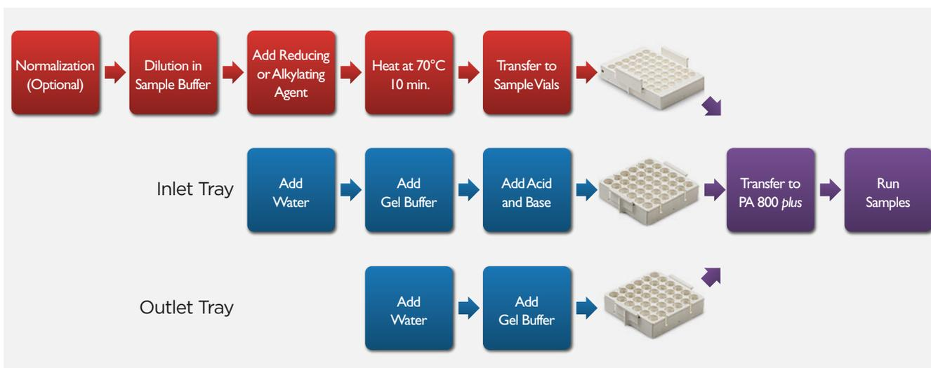
**Figure 2.** Process Workflow. The Biomek 4000 Workstation is used to automate the preparation of samples (red) and buffer trays (blue). The user transfers the sample tray and buffer trays to the PA 800 *plus* and runs the samples (purple).
