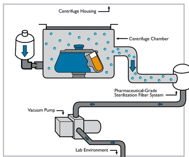
The FRS of the Avanti JXN uses an external vacuum pump to reduce chamber pressure, filtering air from the centrifuge to the lab, all while the rotor is spinning.
