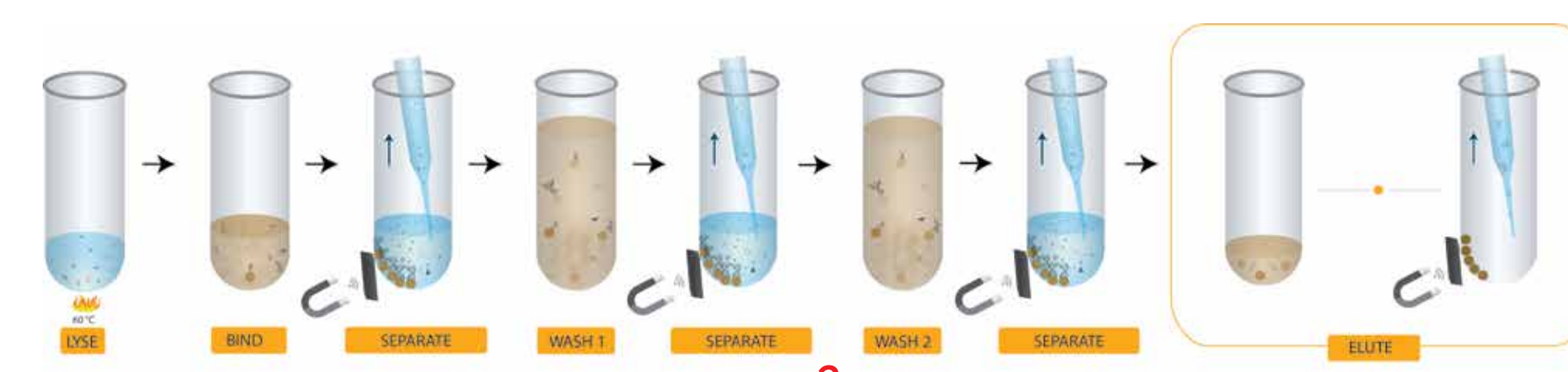
Figure 3. Apostle MiniMax Workflow. The Apostle MiniMax kit involves a lysis step, then the addition of magnetic beads to bind the DNA. Once the DNA is bound, it is washed with various wash buffers and finally eluted from the beads.
