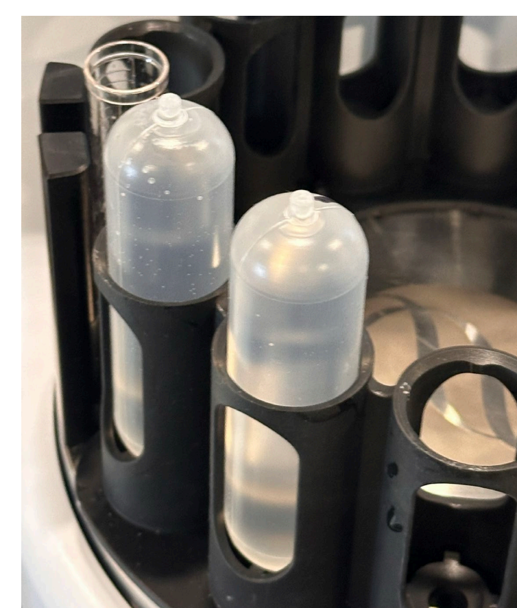
Figure 4. Tubes post-sealing using the OptiMATE system. Produced uniform and reliable tube seal
