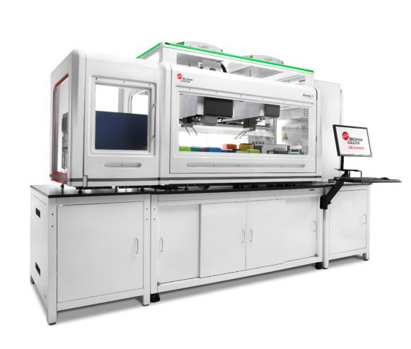
Figure 2. Biomek i7 Workstation. All cell manipulations and sample preparations were performed on a Biomek i7 Workstation with Span-8 pipettors and a 1200µL capacity 96-channel head. A HEPA-filtered enclosure and sterile filtered tips were utilized to maintain cell sterility. The Biomek was integrated with a Cytomat 2C incubator (right), a microplate centrifuge (not shown), and a Vi-CELL XR Cell Viability analyzer (not shown). Cell imaging and protein quantification were performed offline.
