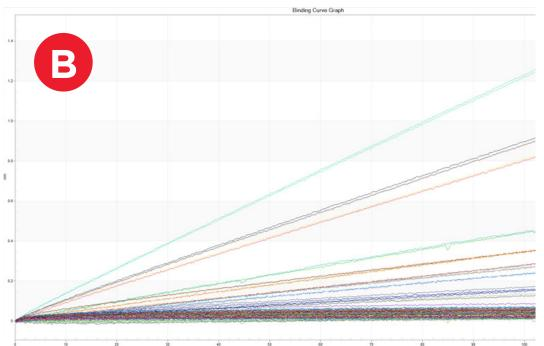
Figure 8. IgG Quantification. A) Binding curves were generated from known Protein A standards (Pall ForteBio). B) Media from wells with clonal growth were assayed for IgG binding to Protein A biosensors. C) IgG concentration was determined for the clonal wells using the standard curve.
