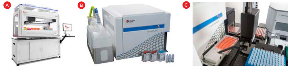
Figure 1. Automated cellular analysis. The Biomek i7 Automated Workstation with HEPA filters (A) was directly integrated with a CytoFLEX Flow Cytometer (B), enabling the Biomek grippers to access the plate loader feature of the CytoFLEX (C).
