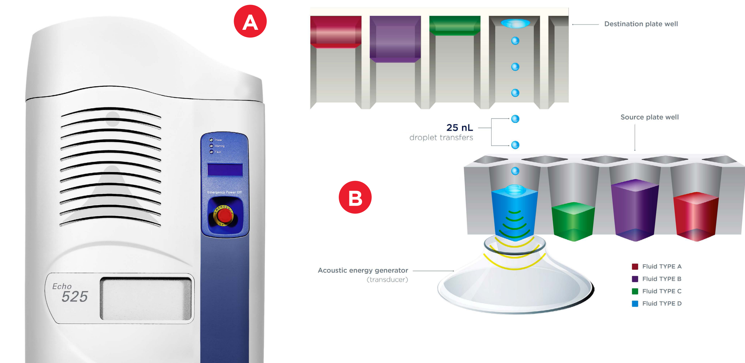
Figure 1. (A) Echo 525 Acoustic Liquid Handler. (B) The Echo system transducer rapidly moves between wells on the source plate while the destination plate also moves, allowing rapid transfer from any well to any well for multiple fluid types.
