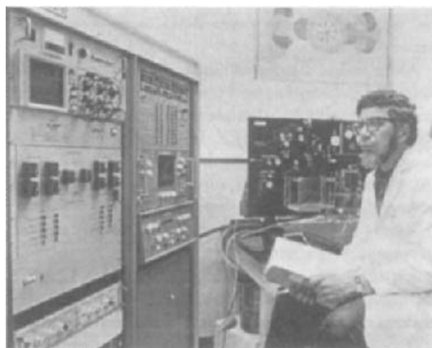
Figure 3-7: Leonard Herzenberg with B-D's first commercial version of the FACS, 1974 (NIH photo).
