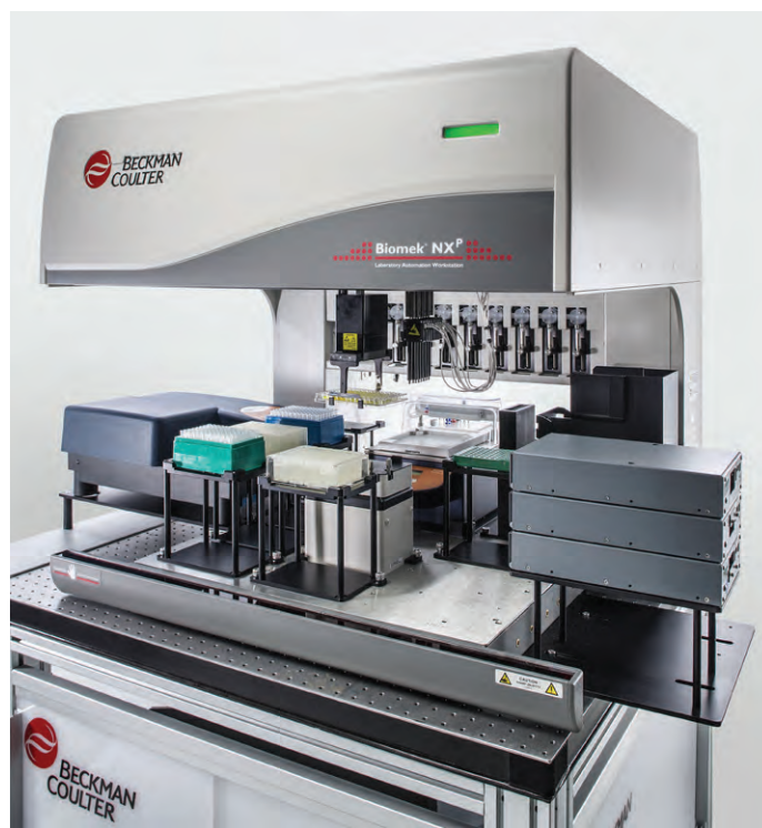
Figure 2. Image of the deck of the Biomek NX P Workstation with the integrated EMax Plus Microplate Reader (left) and the MultiWash+ Microplate Washer (rear, not used for this assay) from Molecular Devices.
