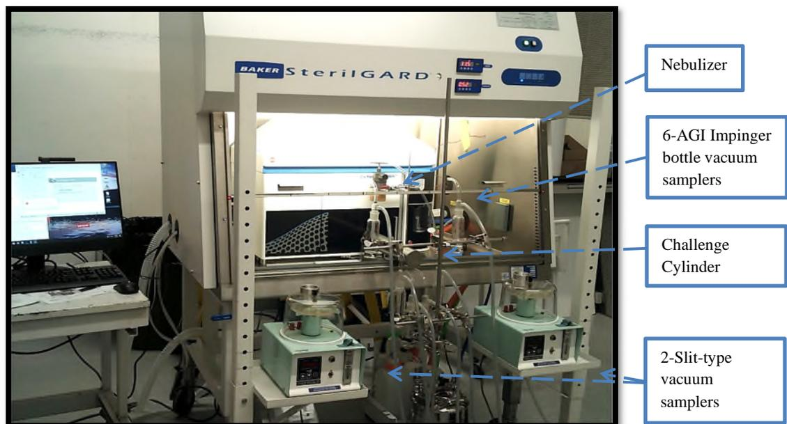
**Figure 3 Personnel Protection Microbiological Test Set Up**
