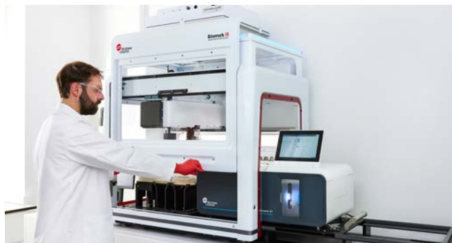
The BioLector XT Microbioreactor and Biomek i5 Automated Workstation integration enables real-time measurement of biomass, pH, dissolved oxygen, and fluorescence—and use these signals to trigger well-specific liquid handling.
