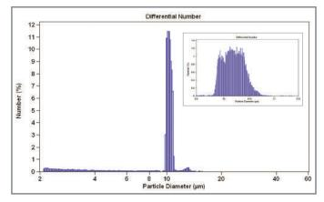
Changes in particle size can be measured in real time thanks to patented digital pulse processing technology. This allows the speed of cell-mediated responses, solutions, aggregates, and dissociation of particles to be analyzed.
