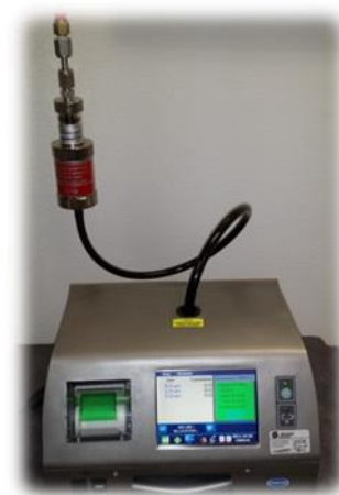
Figure 2 – The MET ONE HPD connected to a MET ONE 3400 series counter and a gas line
