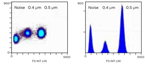
ABOVE: Using the Navios enhanced forward scatter setting, 0.404 micron particles are very clearly resolved from noise, but even more impressive is the resolution of 0.404 micron particles from 0.5 micron particles on forward scatter.
