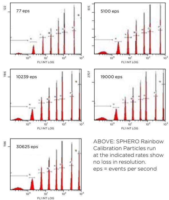
ABOVE: SPHERO Rainbow Calibration Particles run at the indicated rates show no loss in resolution. eps = events per second
