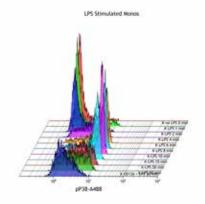
Overlay plots show data from multiple plots on a single pane. Density, dot and histograms can all be utilized in an overlay to easily view trends and changes.
