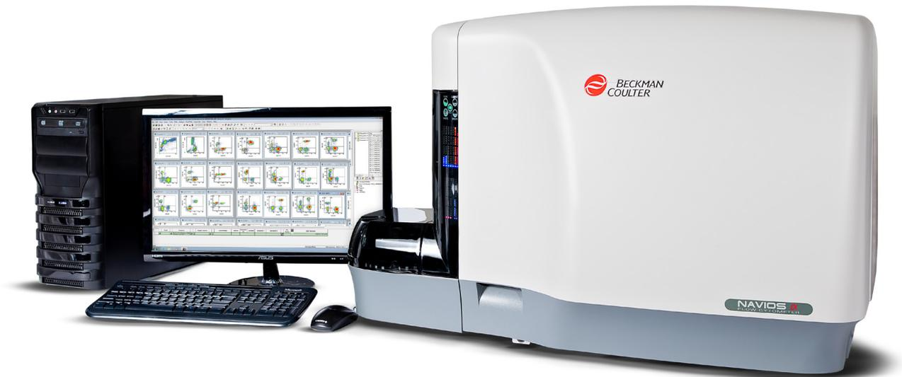
The Navios EX offers up to three high powered solid state, independently-focused diode lasers with an innovative integrated optics flow cell design. Navios EX is equipped with electronics that provide accurate and efficient digital signal processing at high event rates over a wide dynamic range of fluorescence intensities. These benefits are packaged in a compact analyzer that delivers stable performance over long periods of time and across a wide range of operating temperatures.
