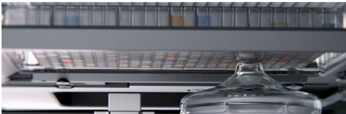
Figure 2: Acoustic transducer moving below the source plate, ready to deliver acoustic energy through the plate and into the liquid.
