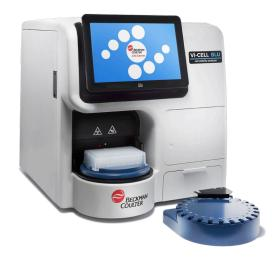
The Vi-CELL BLU analyzer is an industry leading cell viability and counting analyzer that fully automates the widely accepted trypan blue dye exclusion method for cell viability. This analyzer eliminates the historical trypan blue dye exclusion method performed with a light microscope, pipette and hemacytometer.
