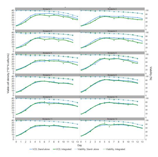
Figure 1. Comparison of integrated (green) and standalone (blue) values on the Vi-CELL BLU cell viability analyzer. The Viable Cell Density (solid line) and viability (dotted line) are shown during the 12- or 13-day cultivation.
