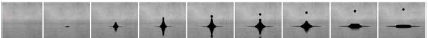
Figure 2: Stroboscopic imaging of Acoustic Droplet Ejection, showing production of a single droplet of fluid.
