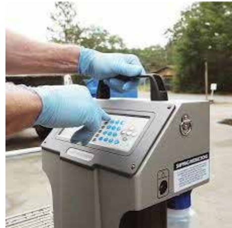
Figure 4. HIAC PODS+ Portable Particle Counter
