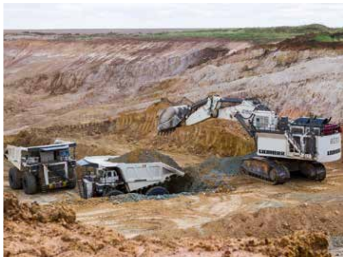
Figure 2. Liebherr R9800 Excavator and dump trucks
