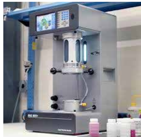
Figure 5. HIAC 8011+ Laboratory Particle Counter
