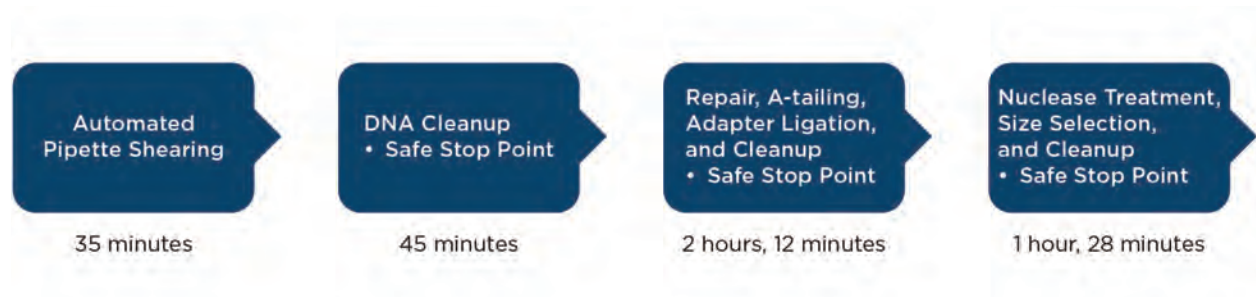
Figure 2. Automated workflow for pipette shearing and SMRTbell prep kit 3.0 on the Biomek i7 Hybrid Workstation. The entire workflow can be processed from start to finish in 6 hours for 96 samples.
