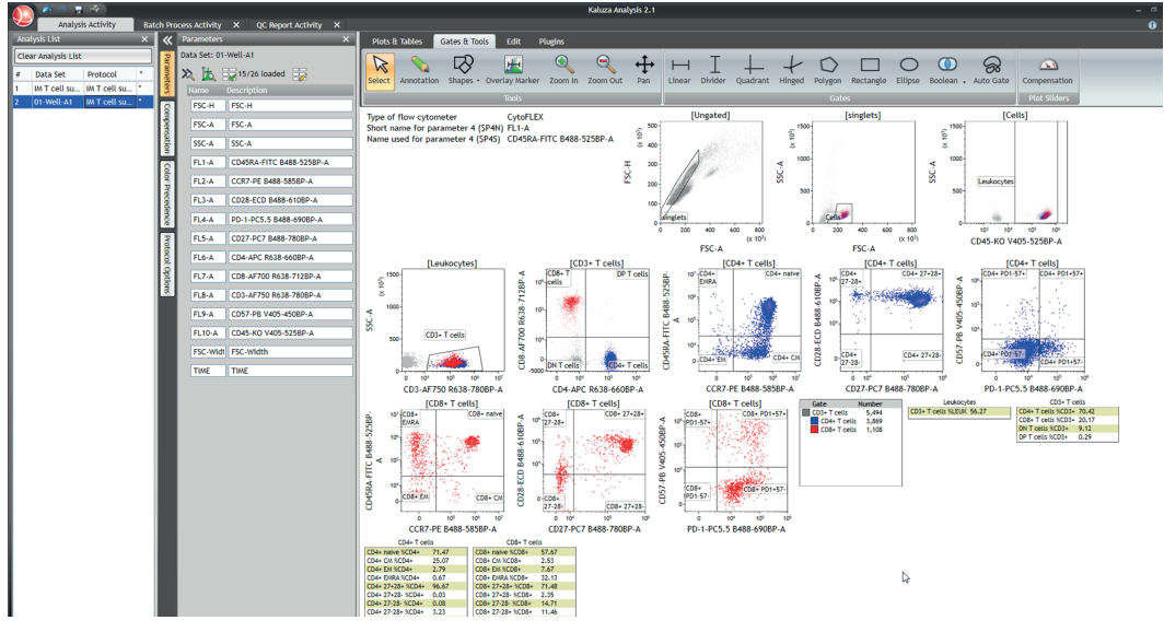
Figure 8. Kaluza Analysis Protocol established on CytoFLEX LX data applied to data acquired on 3L 13C CytoFLEX after scale and gate adjustments.
