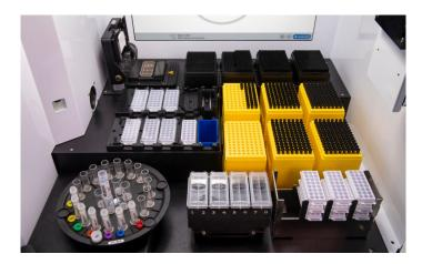
Figure 6. Biomek NGeniuS deck with thermal cycler.
