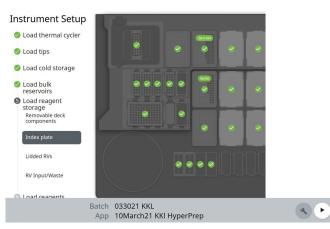
Figure 5. Biomek NGeniuS Dynamic DeckOptix software scans the deck for common setup errors.
