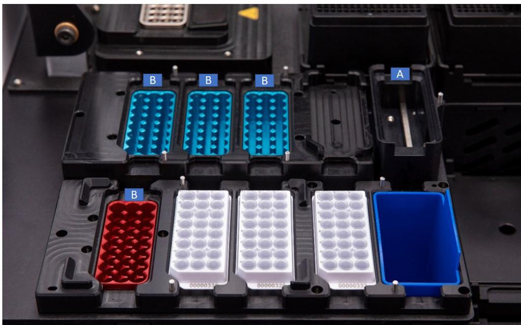
**Figure 7.** Biomek NGenius deck with magnet station (A) and reagent storage zones (B)
