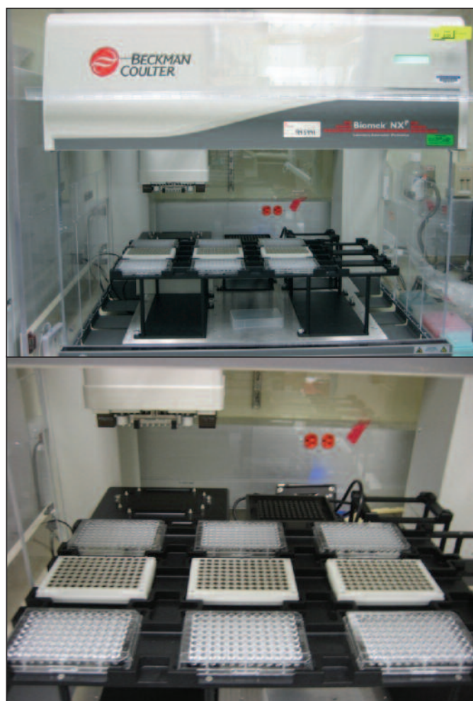
Figure 4. Image of the M.D. Anderson automated HLA-SBT platform on a Biomek NX ® deck configuration for Agencourt AMPure and Agencourt CleanSEQ chemistries.
