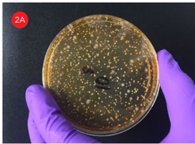
Figure 2. Comparison of the data collection read outs for the Plate Count and Flow Cytometry methods. Panel A is a typical cultured plate from which bacterial colonies are counted. This method requires a technician to accurately discriminate between overlapping or differently sized colonies to obtain counts, typically done in duplicate. Panel B shows the software screen during acquisition using flow cytometry. The instrumentation counts individual bacteria and live versus dead organisms can be differentiated based upon staining characteristics.
