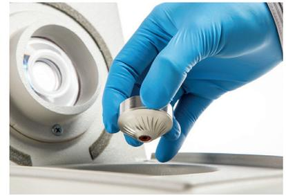
**Figure 1.** The ability of the Airfuge ultracentrifuge to spin small samples at high g-forces makes it ideal for clarifying lipemic samples. Powered by ordinary laboratory air pressure, the ultracentrifuge accelerates to speed in just 60 seconds. Tiny air jets levitate and accelerate the rotor. Turbine flutes machined on the bottom of the rotor provide the driving surface for the air jets.
