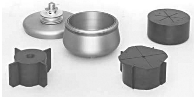
Fig. 6. JCF-Z continuous flow rotor and cores.
