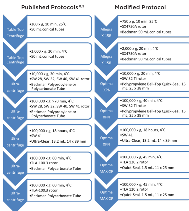
Fig. 4. Comparative protocols showing critical time savings using g-Max technology. Over 1 hour of time was saved in the centrifuge using the modified protocol.
