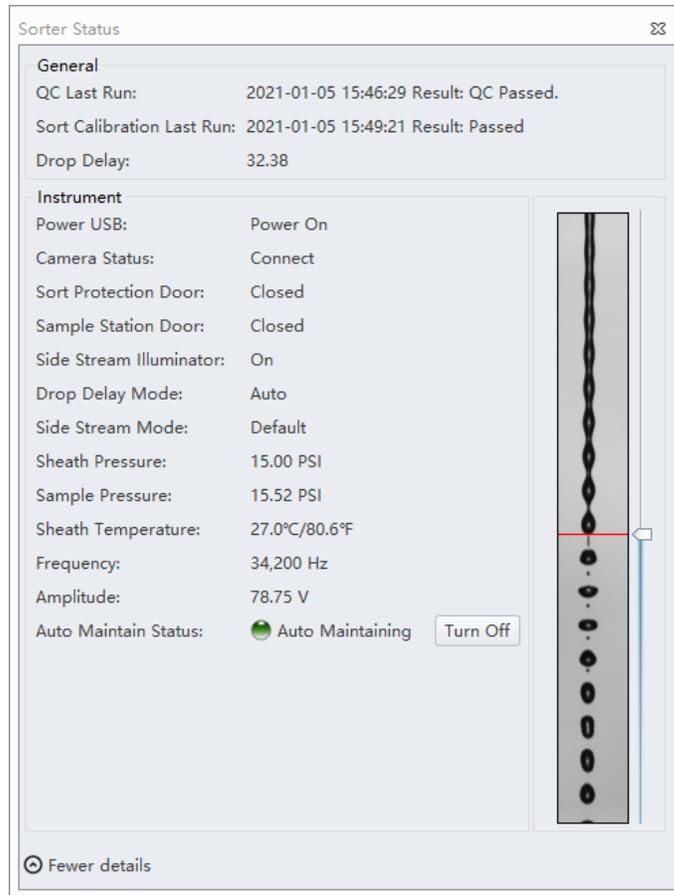
**Figure 1. An illustration of Droplet Formation.** Note the frequency in Hertz, which is also the rate of droplet formation. The last attached droplet is directly above the red line and is the droplet targeted to receive an electrostatic charge.
