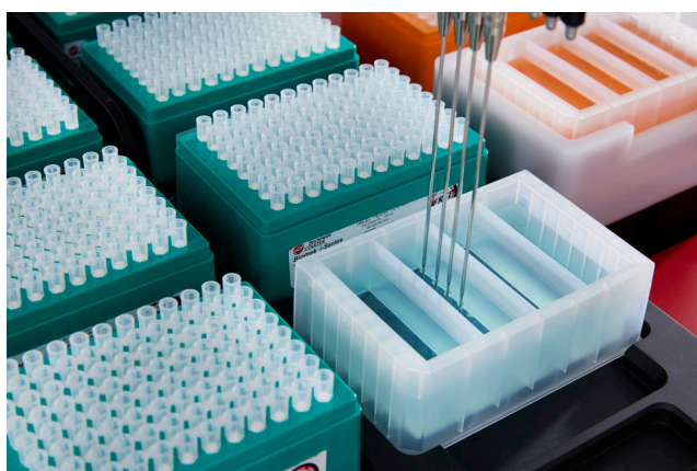
Figure 6. Liquid handler aspirating a culture additive.
