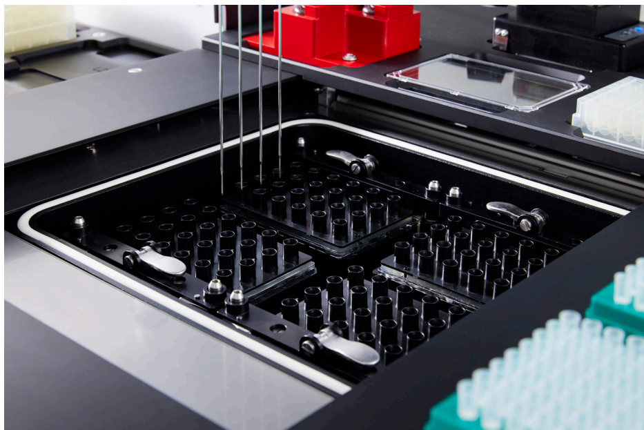
Figure 2. Liquid handler interacting with the bioreactor.
