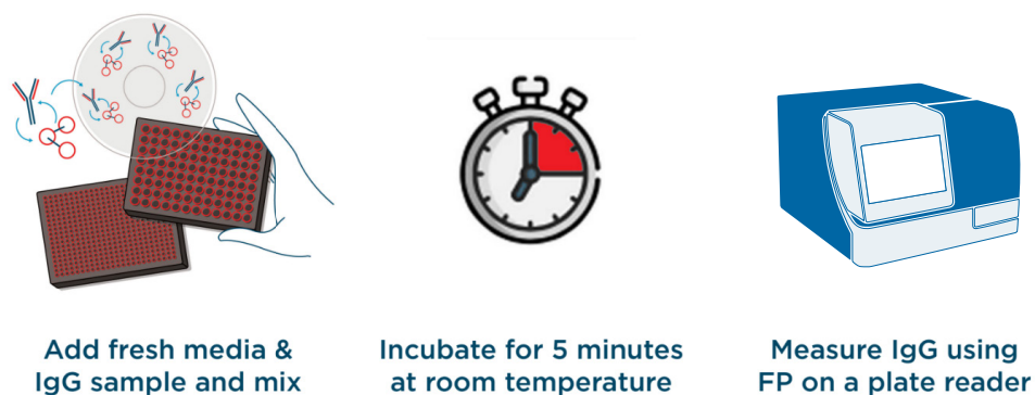
Figure 3: Each well of the assay plate is precoated with a fluorescently labeled Fc-specific probe. An IgG sample binds to the probe. Binding is measured via fluorescence polarization.
