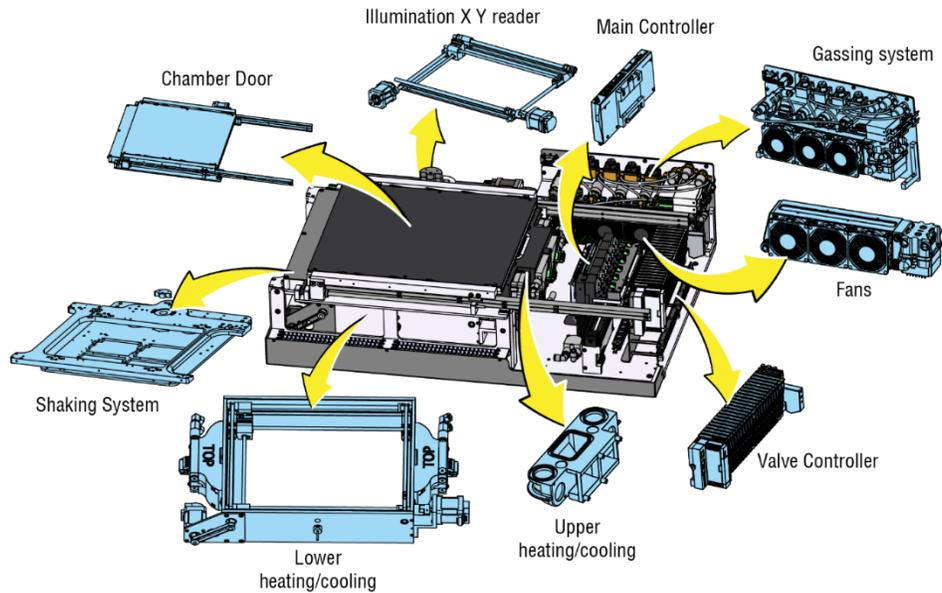
**Figure 1:** Cydem VT Bioreactor module. The bioreactor module provides uniform shaking and temperature conditions. The optical detection system provides in-process monitoring of pH and dissolved oxygen (DO) which triggers  $N_2$ ,  $O_2$  and  $CO_2$  gases to be delivered to individual wells via feedback loops.
