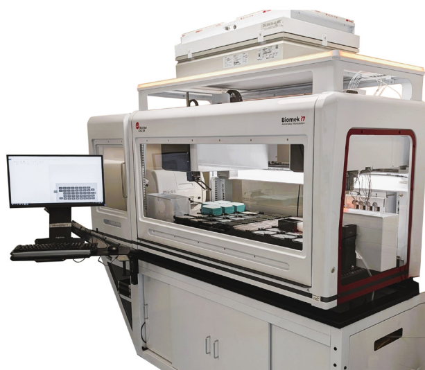
Figure 1. Biomek i-Series Liquid Handling System integrated with a BioTek Cytation 1 Cell Imaging Multimode Reader (Agilent), which creates a seamless flow of data and results analysis.
