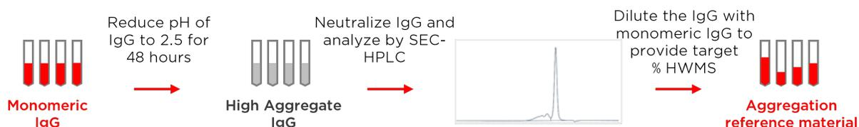
**Figure 4.** IgG is stressed using low pH to induce aggregation and the production of HMWS material. The percentage of HMWS material is assessed through SEC-HPLC and later combined with monomeric IgG of the same parent molecule to provide an aggregation reference material of known % HMWS.
