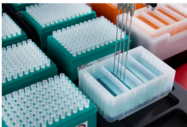
Figure 6. Liquid handler aspirating a culture additive.
