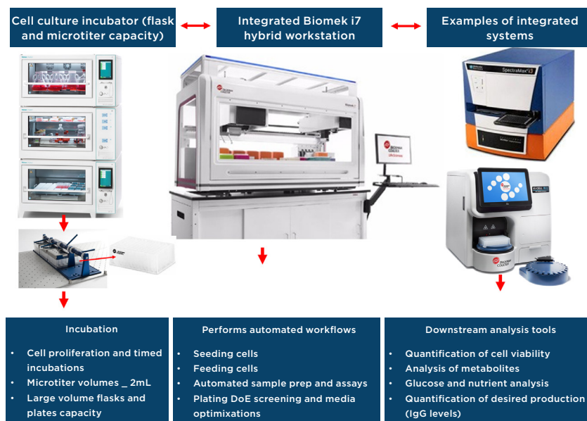
Figure 1. Key technology for development of microplate systems for cell-based process development such as media optimization for IgG development with scale-up potential.
