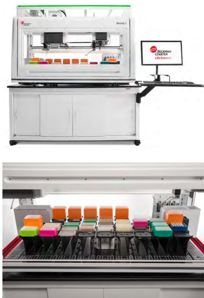
Figure 1. Biomek i7 Dual Hybrid Workstation with optional Enclosure on a Biomek Mobile Workstation. Deck layout in the lower image.
