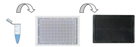
**Echo enabled methods.** The Echo liquid handler uses Dynamic Fluid Analysis to sense differences in surface tension and viscosity in real time. The capabilities allow transfer of enzyme in high concentrations of cryoprotectant, removing a potential error sources and preserving enzyme stability for a longer period of time.
