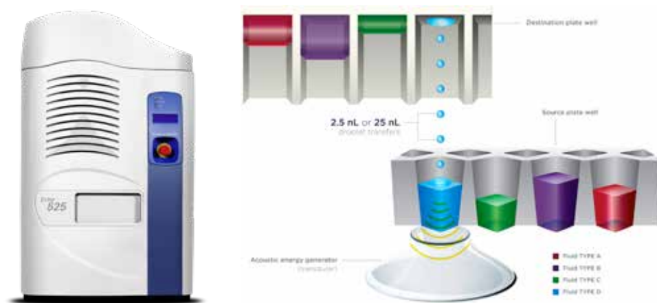
Figure 1. (A) Echo 525 Acoustic Liquid Handler. (B) The Echo system transducer rapidly moves between wells on the source plate while the destination plate also moves, allowing rapid transfer from any well to any well for multiple fluid types.
