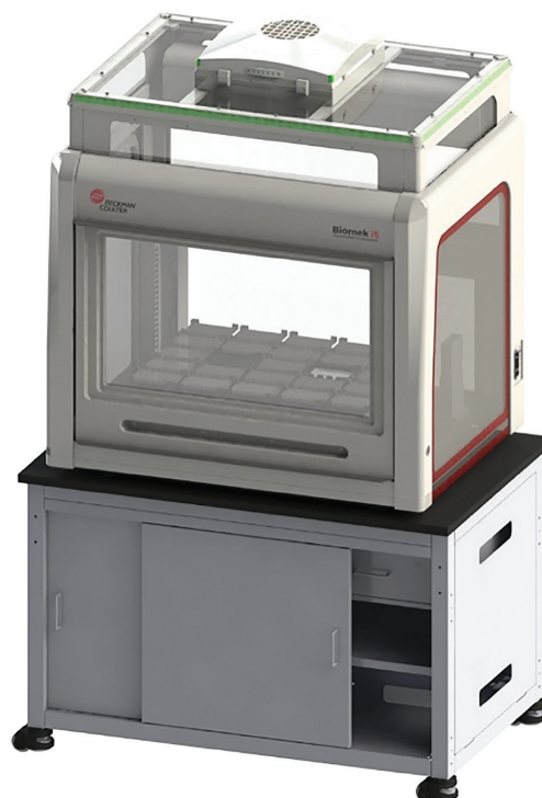
Figure 1. The i5 Multi-channel or i5 Span 8 platform with HEPA enclosure solutions to automate laborious, yet simple, liquid handling steps, such as trypsinization or cell media exchange, of your cell line development workflow process that require traceable and repeatable results in an efficient manner.
