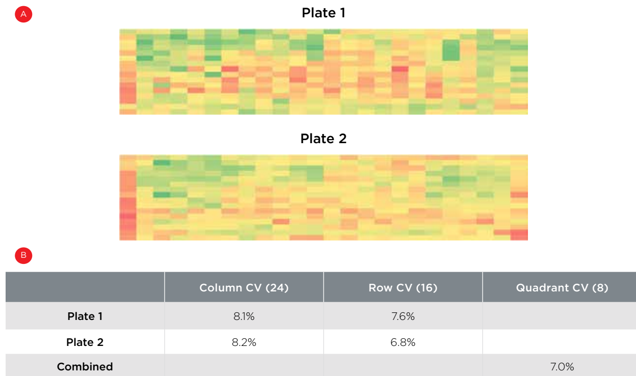
Figure 4. Automated cell plating. A) Heat maps of cell counts in each well of two 384-well plates showing even distribution across the plates. B) CVs of average cell counts across columns and rows for each plate and for the average across the 8 quadrants between the two plates illustrate thorough mixing of cells in the reservoir and consistent multidispensing respectively.
