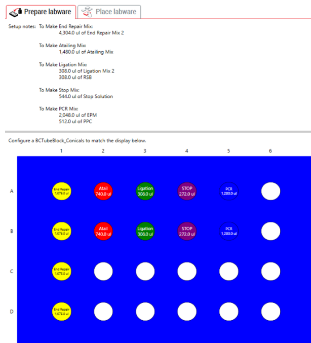
Figure 5. Guided Labware Setup indicates calculated reagent volumes required to make reagent mixes and guides the user for correct deck setup
