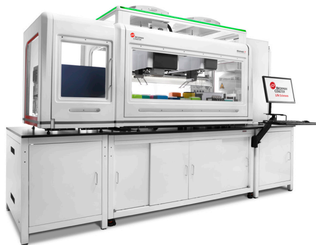
Figure 1. Biomek i7 Workstation with integrated devices to enable cell line development/cellular applications.
